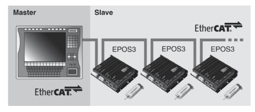
The EPOS3 70/10 EtherCAT is a modular, digital positioning controller and suits DC and EC motors with incremental encoder in the range up to 700 Watt.
